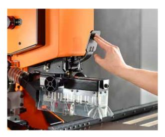
Save time and money – improved setup and compatible tools MINIPRESS top employs a new tool-free clamping technology which makes it quick and easy to change drill heads. You can also use the drilling heads and rulers of PRO-CENTER and MINIPRESS PRO. The comprehensive modular system of drill heads and rulers allows you to tailor MINIPRESS top to your manufacturing requirements.
