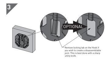
Hold the component in place and fasten to the substrate/ surface with 8G screws. Repeat for matching component. Ensure sufficient screw embedment in substrate. IMORTANT all screws must be flush. IMPORTANT NOTE: Prior to assembly, establish whether the joint is to be permanent or will need to be disassembled. If it is to be disassembled then remove the locking tab.
