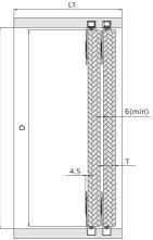
W = door widthL = wardrobe internal width Door width: W = L/2 + 15Door self-closing distance k=50
